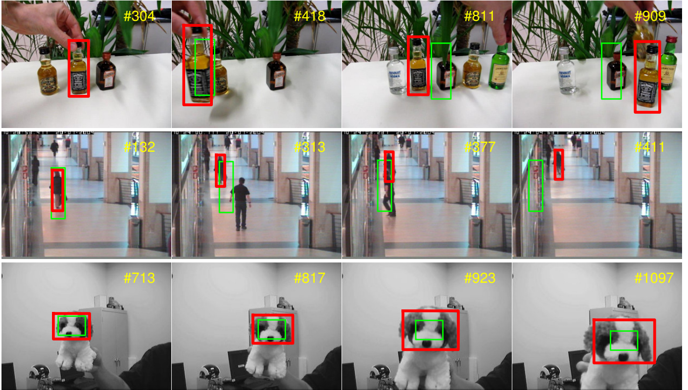
Fig. 1. Comparison of our discriminative scale space tracker (in red) with the standard DCF based translation tracker (in green). Example frames are shown from the liquor (top row), walking (middle row) and dog (bottom row) sequences. The standard DCF tracker is not able to handle the scale changes in these sequences. In contrast, our approach accurately estimates the target size, thereby significantly increasing both the accuracy and robustness of the tracker.
