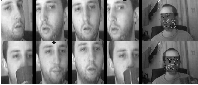
Figure 3. Four modes of the learnt appearance model for head tracking represented by medians. Also shown is the state of the tracker. Top: The head has rotated and translated and various modes of rotation have been separated out by the model allowing view specific predictors to be learnt for each aspect of the head. Bottom: Occlusion introduces a new appearance cluster but after occlusion is over an existing mode of the appearance model with all its associated predictors is reactivated. The black mark indicates which component to be used next. The left most images show the tracker output and the linear predictor placements, white predictors are currently active and black ones are inactive.
