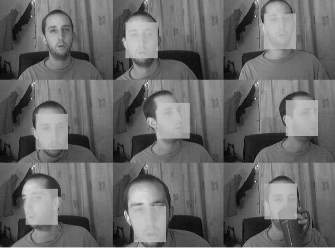
Figure 4. Prototypical results from tracker running at between 20 and 25 frames per second. Tracking through large pose variations and over 100 frames of occlusion
